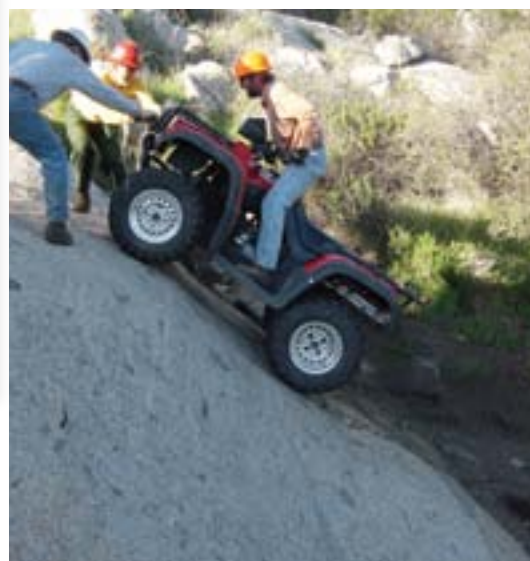
This is a durable natural feature, but where is the line between challenge and risk? If an ATV is the design vehicle, utilizing this feature may have crossed it. This does not look that difficult, but poor soils or poor sight distance due to the alignment may have prevented getting a run at it.
