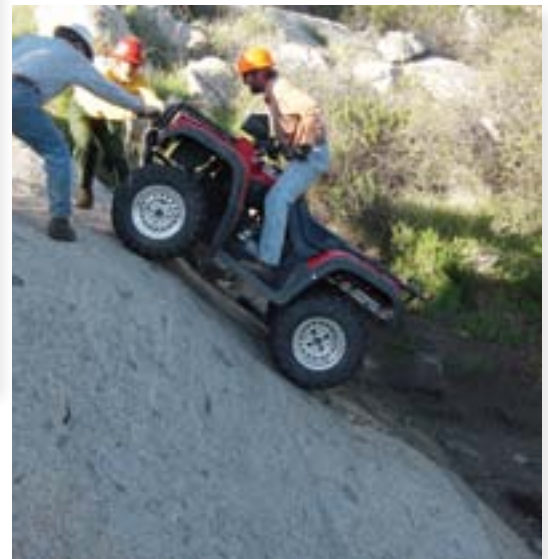
This is a durable natural feature, but where is the line between challenge and risk? If an ATV is the design vehicle, utilizing this feature may have crossed it. This does not look that difficult, but poor soils or poor sight distance due to the alignment may have prevented getting a run at it.
