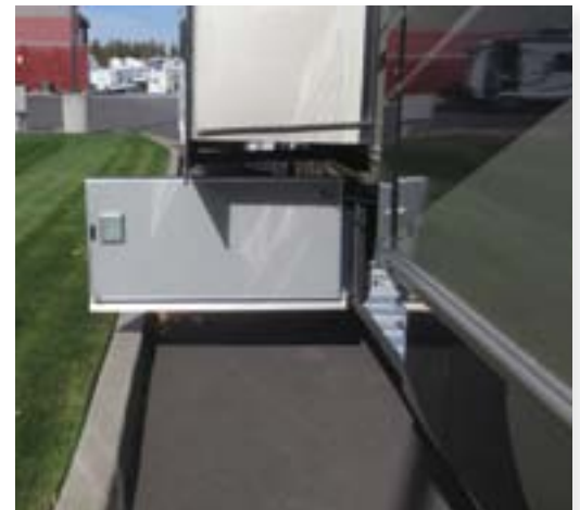
This slideout extends 36", but the storage bay door extends 52". Trees, bollards, or logs used to define the site can also restrict its use with inadequate lateral clearances.
