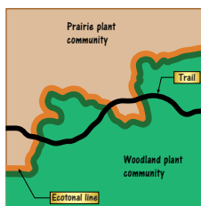
Cross the same edge repeatedly: Creates dynamic excitement and feeling of rapid change, feels well integrated into the site
