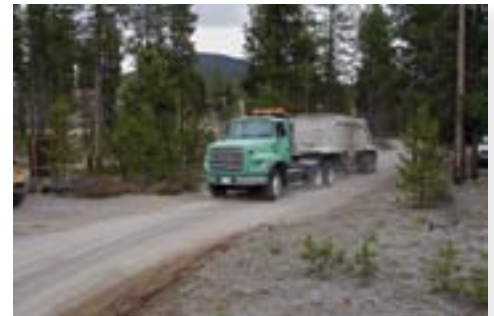
The belly dump truck makes a good test vehicle for roads and spurs in a big rig OHV facility.
