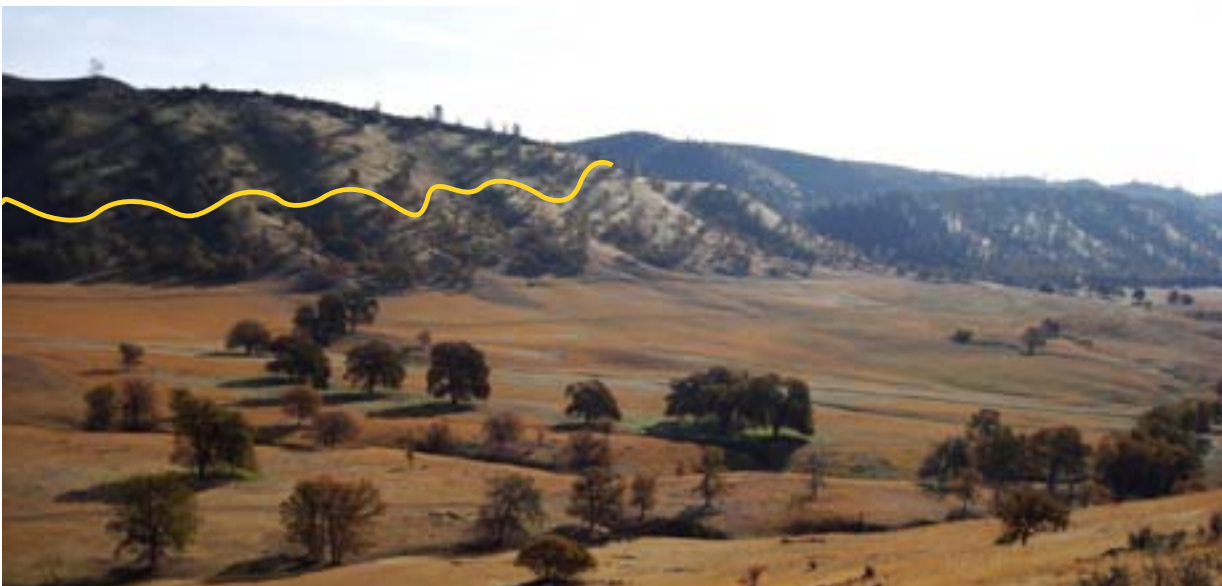
Locating a fun, sustainable, and visually unobtrusive trail on an open landscape can be challenging. Note the undulating W shape of this location. If nothing else, this trail will drain well.
