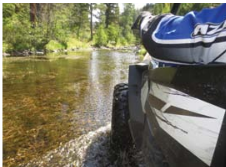
Flat water and a gravelly creek make this a better crossing, but it's longer than it needs to be because it is not perpendicular to the creek.
