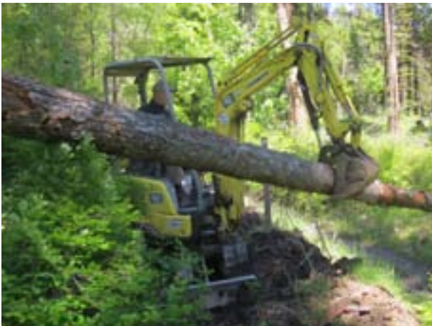
A bucket with a thumb is great for grabbing material and placing it strategically without a lot of ground disturbance. The versatility of a mini-excavator makes it a good choice for finesse or finish work.
