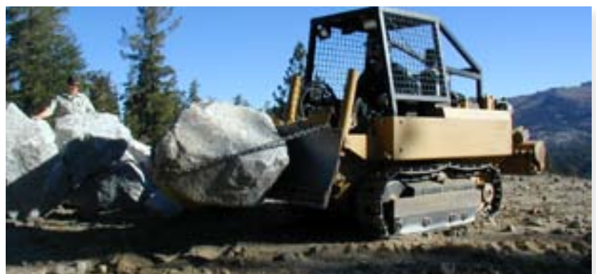
A 6-way blade makes short work of trails on steeper ground.
