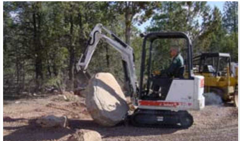
The ability to work on steep slopes, scatter debris and reach down to remove woody debris from the embankment area is an advantage.
