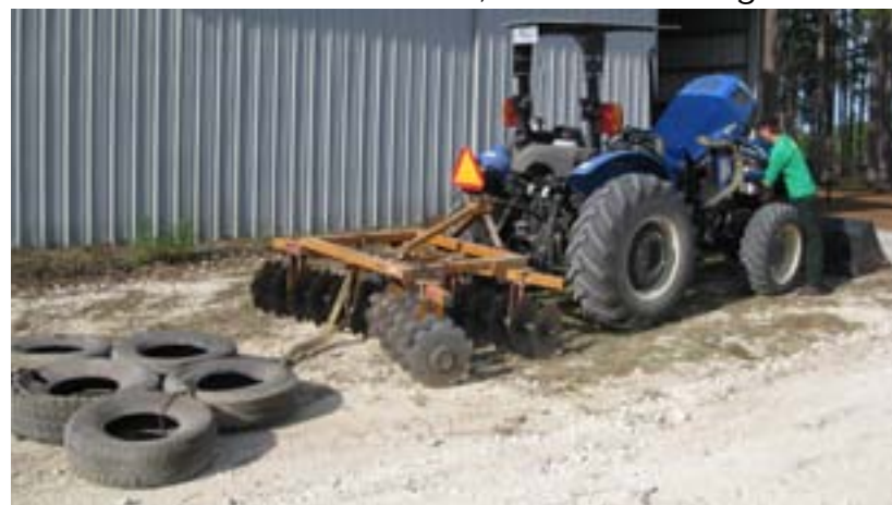
This disc and tire combination is being used on sandy trails. Due to its length, this unit would not work well with a tight curvilinear alignment.
